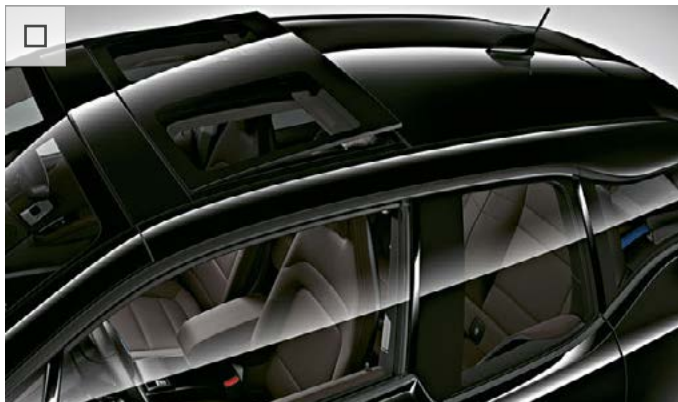
The electric glass sunroof features sun protection glass, tilt and slide function and an integrated wind deflector.
