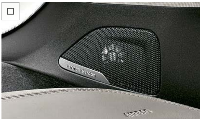
The harman/kardon loudspeaker system with surround mode has a 360W digital amplifier, vehicle-specific equalising and 12 speakers.
