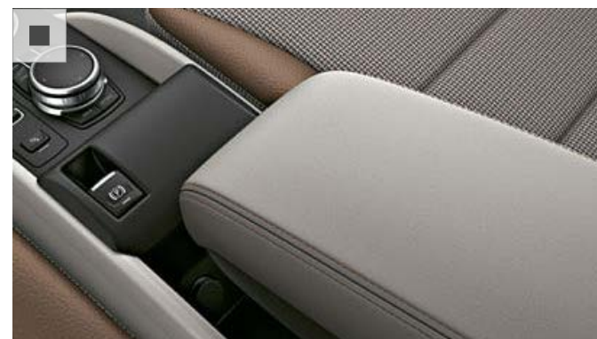
The folding front armrest has three positions and includes an integrated storage compartment.
