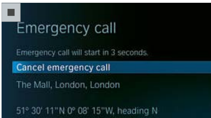
BMW Emergency Call automatically establishes a voice connection with the local emergency services without the use of a mobile phone. It also transmits additional information such as the vehicle's current location. BMW Emergency Call can also be triggered manually in case other road users require help.
