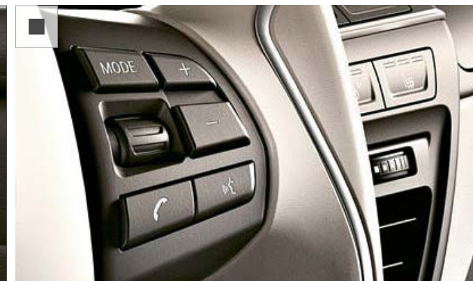
The multi-function buttons for the straps and cupholders. steering wheel can be used to operate the telephone settings, audio and Cruise Control.
