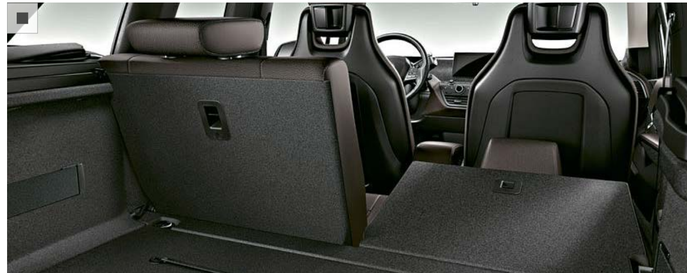
The backrests can be folded down in a 50:50 ratio and each side can be set to one of three positions, as required.
